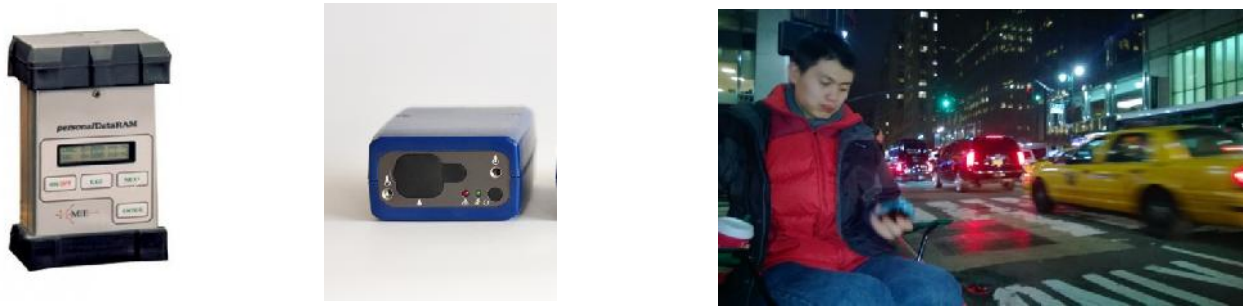
Figure 4 –Air Quality Monitors (left) PM2.5 monitor MIE PDR 1000, (center) BC monitors microAeth® Model AE51, (right) William measuring street level air quality
