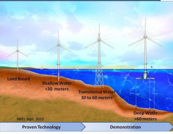
Starting with shallow, fixed foundations, moving to floating foundations.
